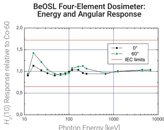
The four-element dosimeter has two additional detectors; one is covered with copper and the other one with lead. These detectors receive information on energy. This means our algorithm can deliver a higher accuracy and clearer information on the irradiated radiation quality compared to other dosimeters.
